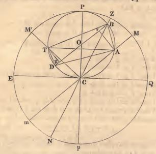
a terrestrial meridian; P, p, the poles of the earth; E Q the equator; (Z) the zenith; (N) the nadir of a place on this meridian; M the place of the moon. Then
